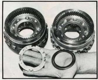
A similar needle bearing is used in rear planetary output carriers (shown here) and forward clutch drive hub.
