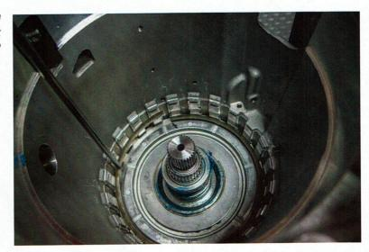
This is a factory snap ring on top of a Super 80 snap ring. The Super 80 snap ring is both larger and thicker that the factory GM. The outside edge of it fits into a groove that is machined into the case in the top half of the lugs section.
