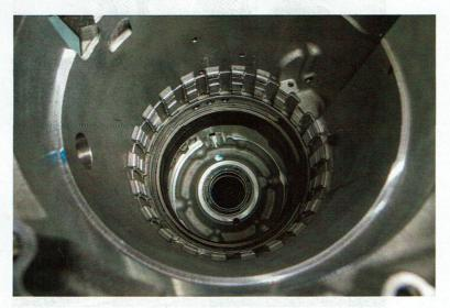
This is the inside of the Super 80 case. The lugs cover the full 360° circumference of the case. The Super 80 case is not only better by design, it is also formed using a better casting process for increased strength over stock cases. GM cases are die cast which uses different alloys than permanent mold casting which is how Reid casts their cases.
