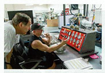
Jim and Dennis watch the gauges on the dyno while it is run though all of the gears. Like most of the specialty tools and equipment at ATO, Jim designed and built the dyno himself. The dyno gives Jim the ability to fully test every function of the transmission and torque converter without installing them in a car. When the customer picks up a transmission from ATO they can be confident it is race ready.
