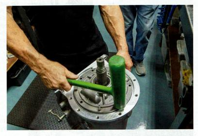
On the bench the transmission is flipped over so Jim can install the ATO full manual/fully mechanically controlled valve body. Then the filter, pan, bell housing, and torque converter are installed.
