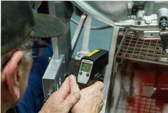
While the transmission is being run on the dyno Jim checks operating temperatures at multiple locations.
