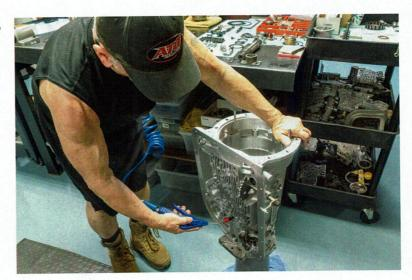
Then the band that actuates the 2nd gear compression braking is installed. Jim modifies this band in house by welding two parts of the band housing that are riveted together because he has seen the rivets fail.
