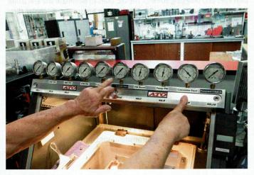
While running the transmission through all of the gears, Jim watches the gauges to make sure the valve body works perfectly.
