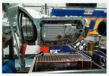
After Jim has given the transmission a full test on the dyno, the pan is removed to drain the fluid and the transmission is ready for installation.
