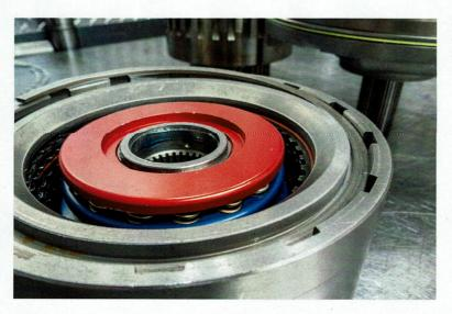
This is the direct drum and its return spring retainer. The springs disengage the clutches quickly when downshifting from 4/3 to 2nd to reduce drag. Jim uses an upgraded aftermarket assembly that has upgraded springs.
