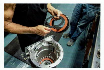
After the snap ring is installed the intermediate clutches that actuate 2nd gear are installed.
