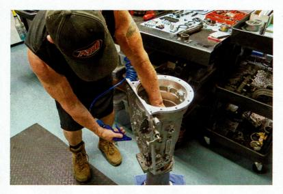
Jim air tests the direct drum then installs the forward drum. and back half of the overdrive assembly.
