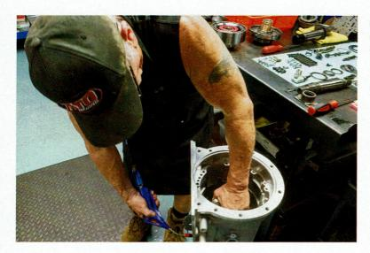
Jim used a custom made tool to install the direct drum. The tool is put in place of the direct drum pressure plate with the snap ring 3/4 installed for ease of removal and then he lowers the assembly into the case. Once it's in the case the snap ring is pulled out so the tool can be removed and the actual pressure plate is installed followed by the snap ring.
