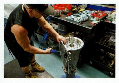
The turbine shaft, housing assembly, and overrun clutch are then installed and bolted in place from the bottom of the case. The circuit is then tested with air for proper function.
