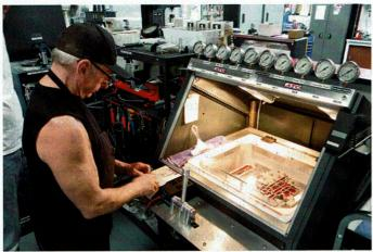
Jim built his own valve body testing dyno so he can test all of his custom built valve bodies without putting them in a transmission. It monitors pressure in 10 places and can be run through all gears.
